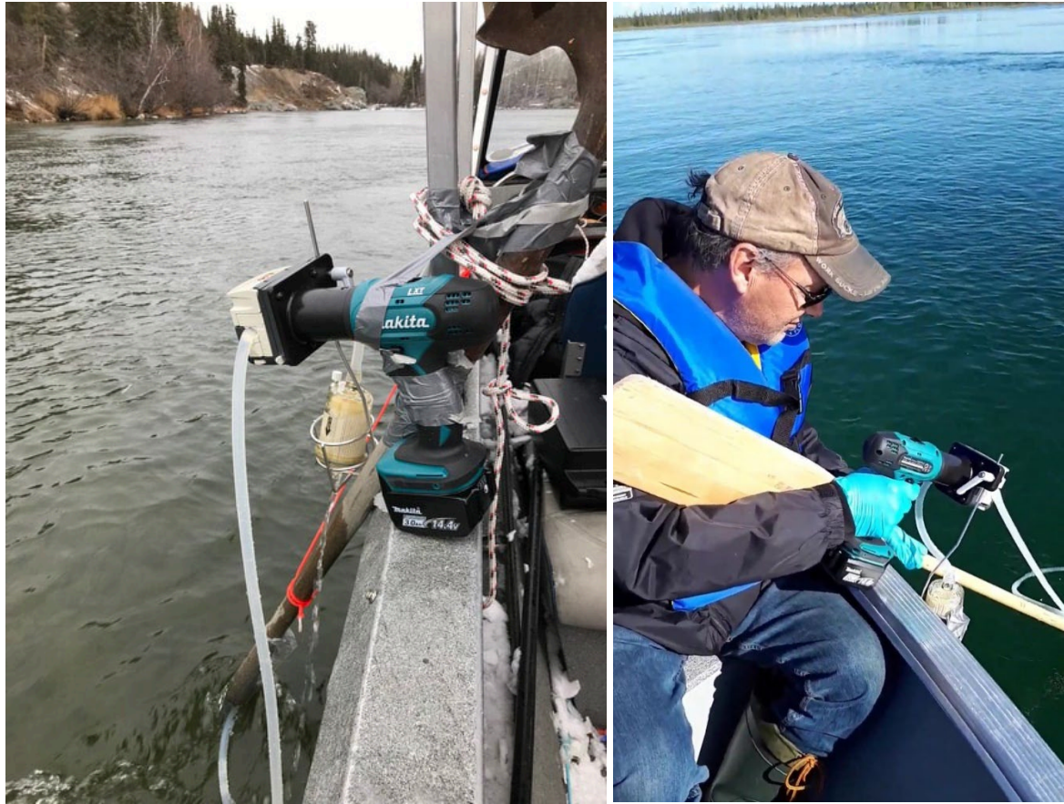
Figure 5. River samples (lotic) taken using a modified drill made by SPYGEN, which pumps water through the filter capsule by the power of the peristaltic pump on the drill head. In both events, the samplers uses paddles to ensure the filtering tube remained underwater for the duration of sampling.
